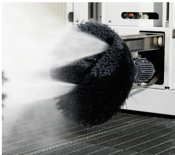
**Wheel Master** is the system designed for washing the vehicles' tyres, sides and underside.
