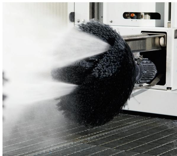
**The Wheel Master** is developed to wash the wheels, the side of the car and all lower parts of the vehicles. Operated by **two high pressure nozzles**, thanks to a great combination between power of the high pressure and the softness of the brush, Wheel Master guarantees an **excellent washing result even in difficult spots**.
