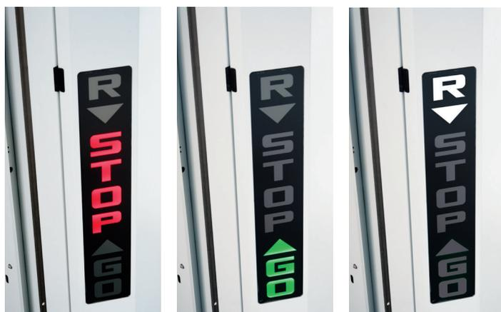
The **display on the columns** of the machine adopts backlit icons to easily drive the client exactly in position to start the washing cycle.
